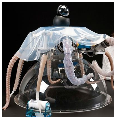
Figure 10. Soft-armed/legged robot for multi-point flexible and secure gripping [from Laschi, 11]
