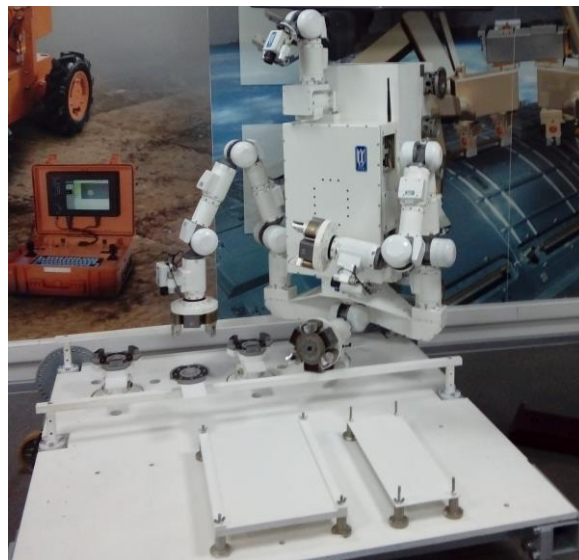
Figure 9. RTC Multi-axis, multi-arm, self-interchangeable gripper-manipulator robot (ISS selection)
