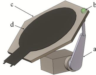
Fig. 4: Elements of “feather”. a – servo, b – light-emitting diode (LED), c – base, d – force-sensitive resistor.
