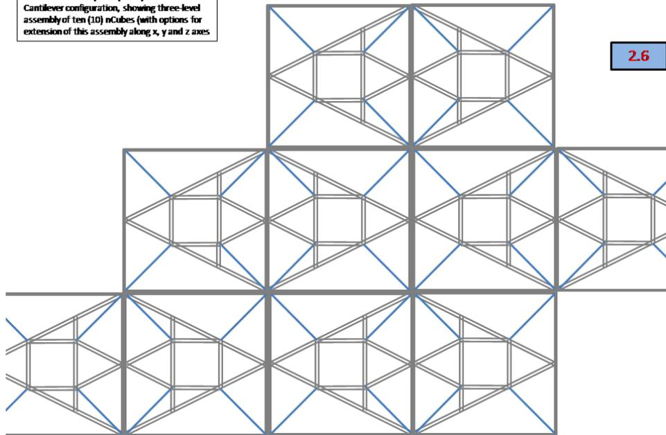
Figure 10 – Combining Alpha and Cantilever elements for large multi-level PodAtriums
