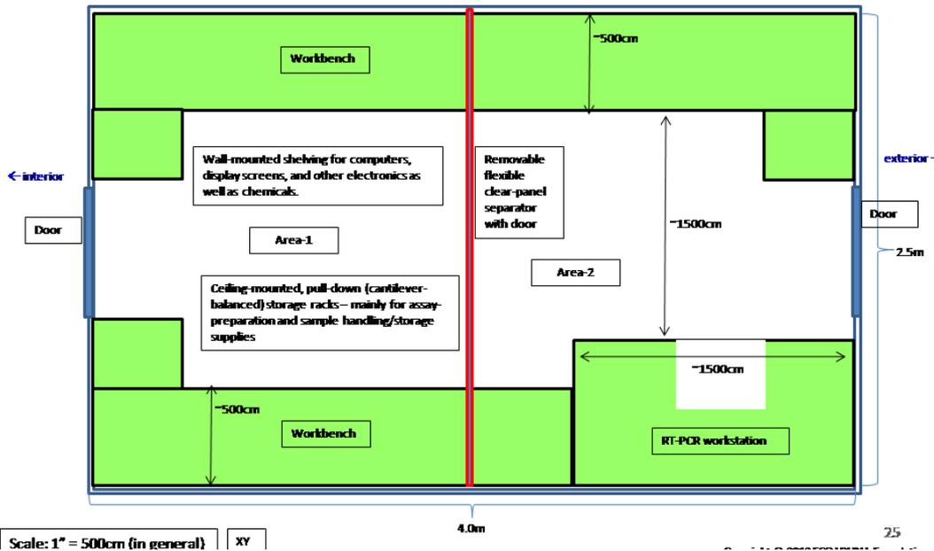
Figure 12 – BSL – Biological and Chemistry Laboratory/Workspace nPod
