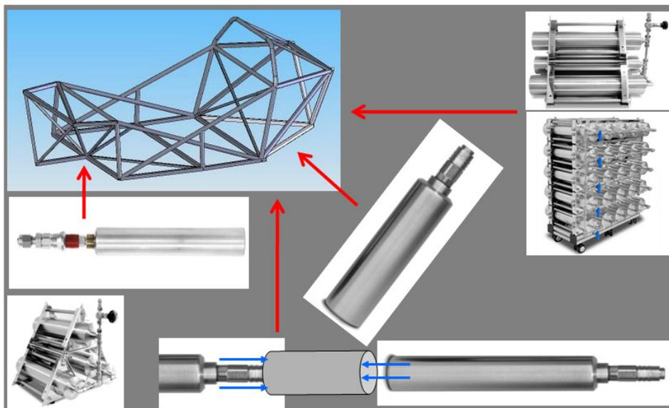
Figure 15 – Hydrogen Fuel Cell Storage and Generator Units - as nPod Structural Elements
