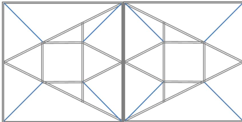
Figure 9 – Two Alpha elements make a cantilever structure for multi-level nPod complexes
