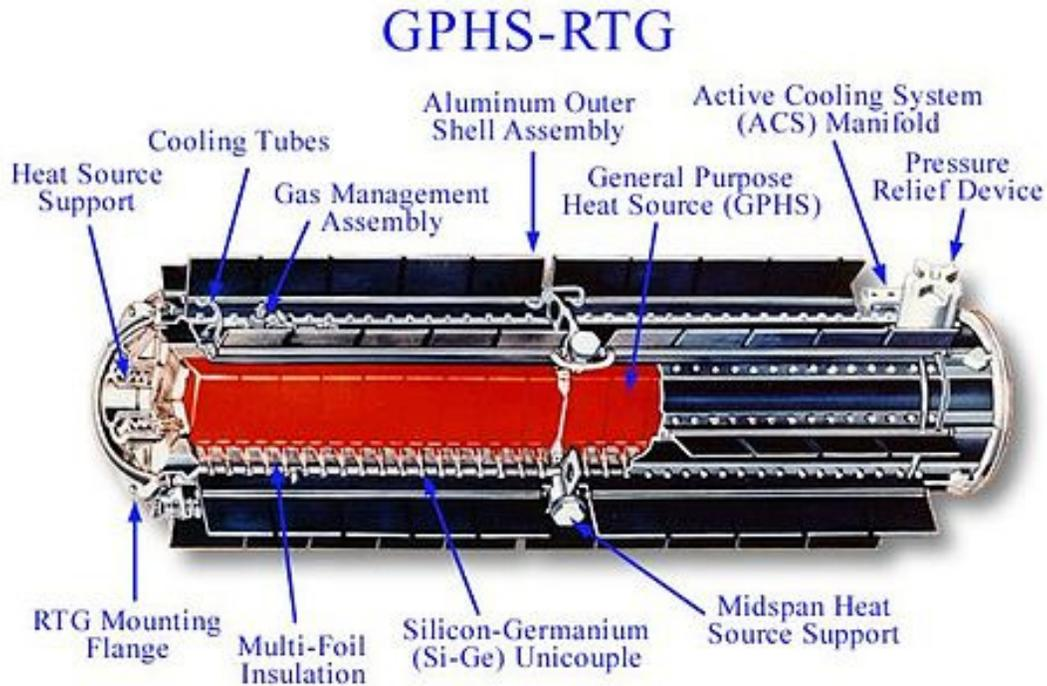
Figure 16 - RTG – Radioisotope Thermoelectric Generator – as an nPod Structural Element
